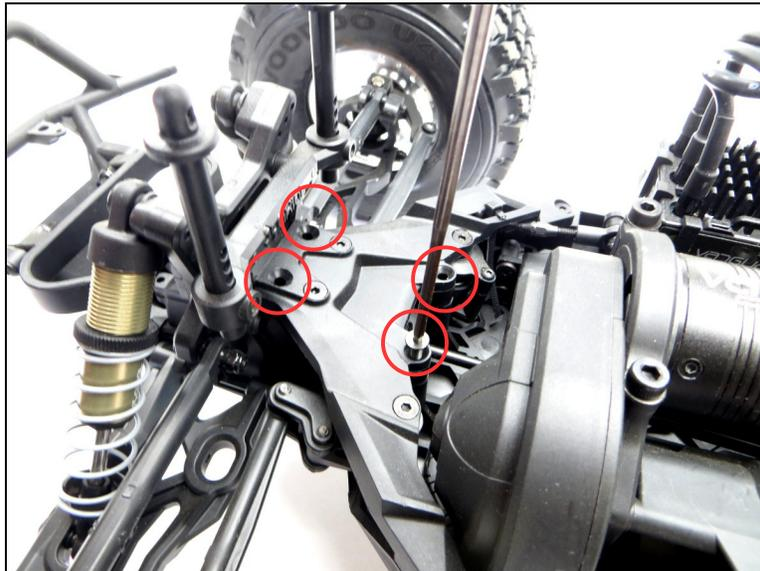
4. Install WINCH PLATE with 3Racing Winch using the (2) M3 x 14mm and (2) M3 x 20mm Button Head Screws as shown (M3 x 14mm in the front two positions and the M3 x 20mm in the two rear positions):
