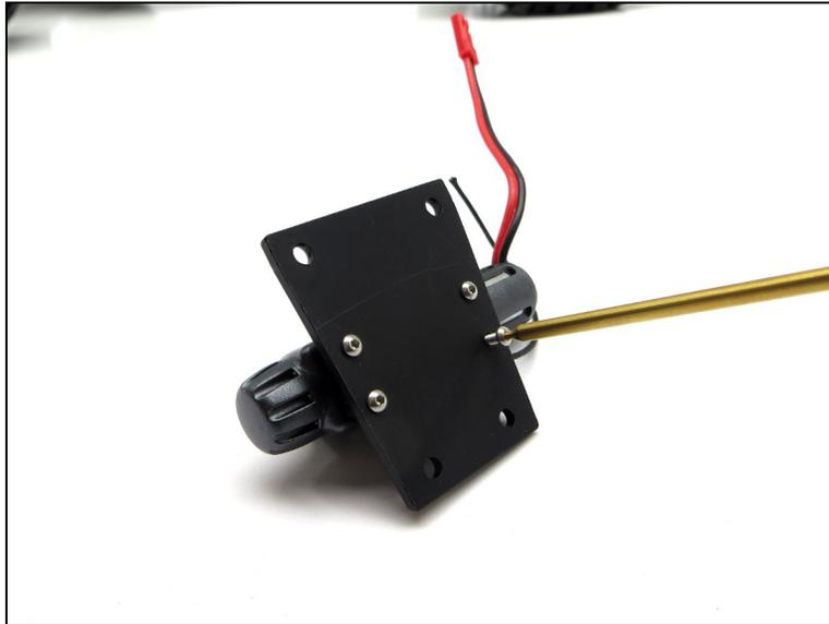
3. Remove the (4) flat head screws from the Yeti as shown:
