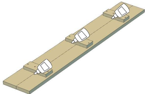
5. Remove and glue Legs (D) to Table Ends (F), making sure the laser-engraved line faces away from the glued area (see illustration). You will build two table ends.
