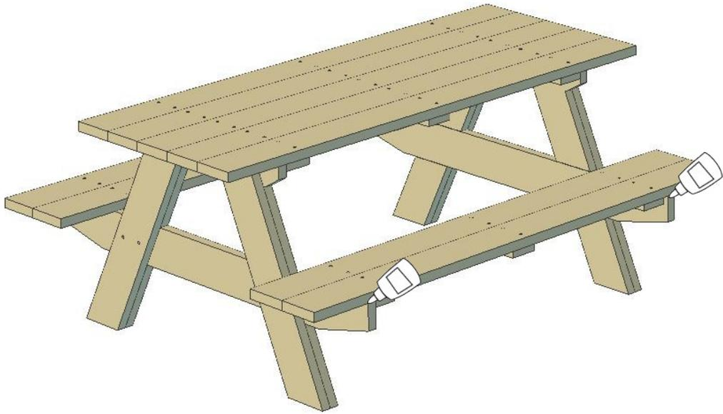
8. Remove Braces (E) from sheet and glue to bottom side of Top and inside the Leg Assemblies as shown.
