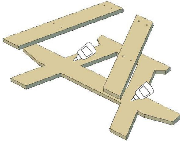
6. After glue has dried, glue two Leg Assemblies to the Top as shown.
