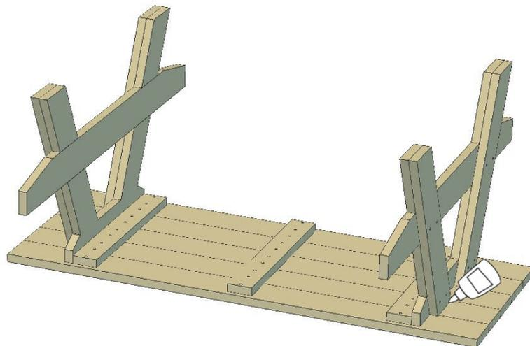
7. Glue two assembled Benches to the Leg Assemblies.
